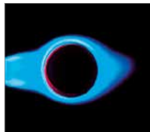
High flame temperature based on cyclone swirl
