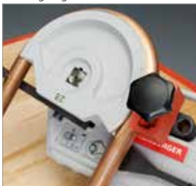
Forged aluminium segments with bending angle scale
