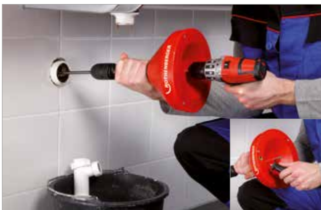
Electrical operation with cordless drill
