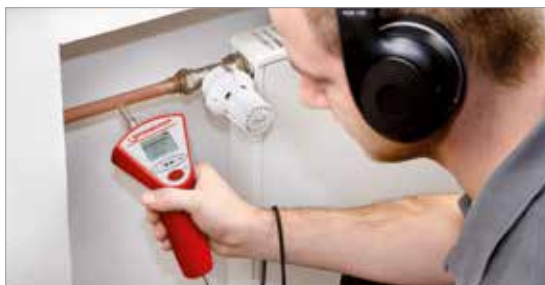
Acoustic leak detection of heating installations
