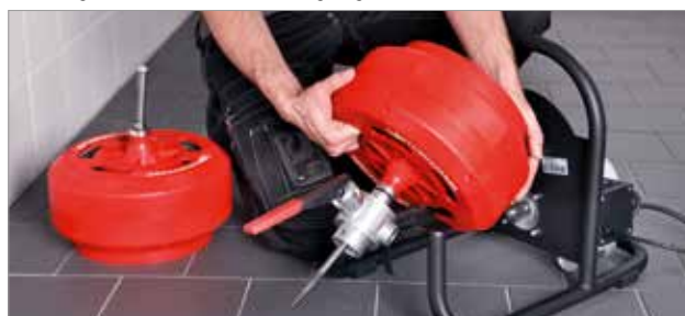
Interchangeable drum for different working ranges
