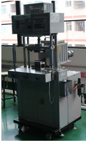
Low Temperature & Lower pressure molding for cable with PCB or Chipset
