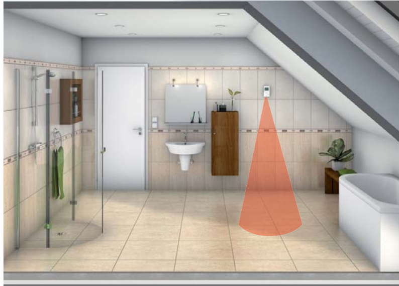
Infrared measurement of the surface temperature establishes the optimum temperature to keep feet comfortable
