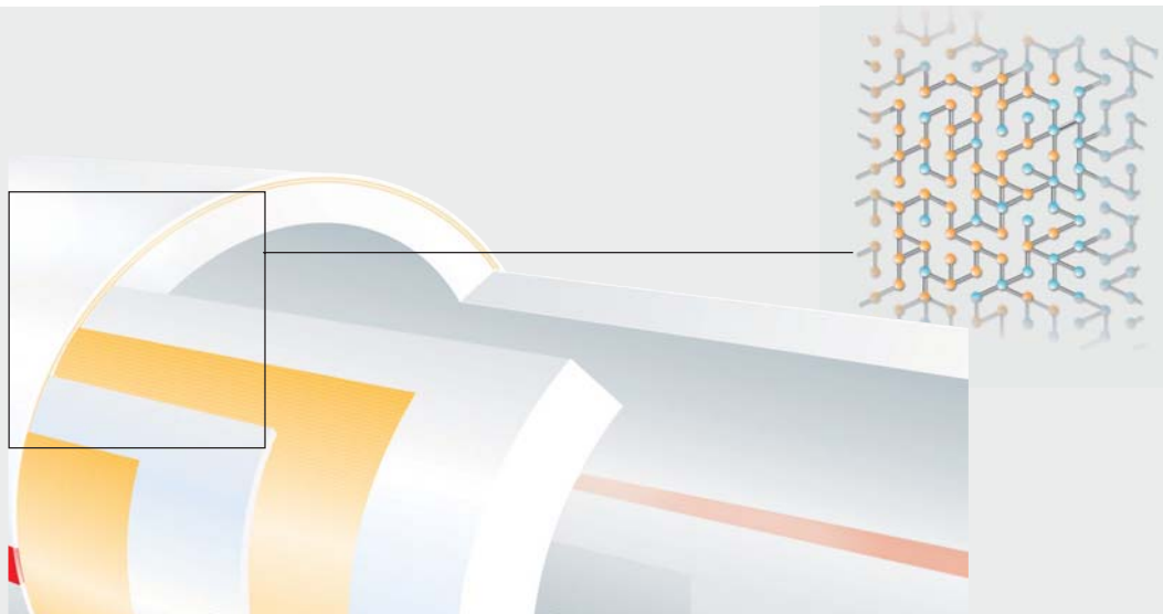
All five layers of the Roth DUOPEX S5® System Pipe are co-extruded and then cross-linked.
