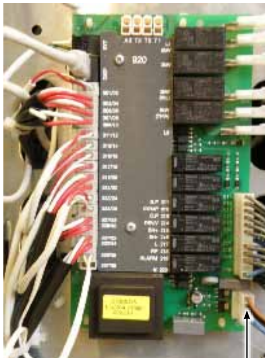
The voltage for the HGW shunt is measured here
