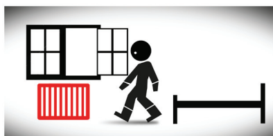
Fresh, cool air flows in and is detected by the living connect ® thermostat; shortly thereafter the radiator is certain that the window is open , and the thermostat will then shut off the heat.
