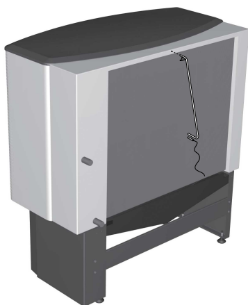
Figure 11. Hook the defroster sensor mounting into place
