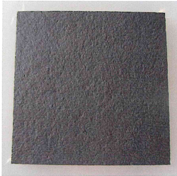
Photo 1: Material Insul sheet/ roll 6mm, color black: fungal growth was not visible to the naked eye
