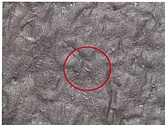
Photo 2: Material Insul sheet/ roll 6mm, color black, color white: (at a magnification of x 50): low fungal growth was visible under the microscope
