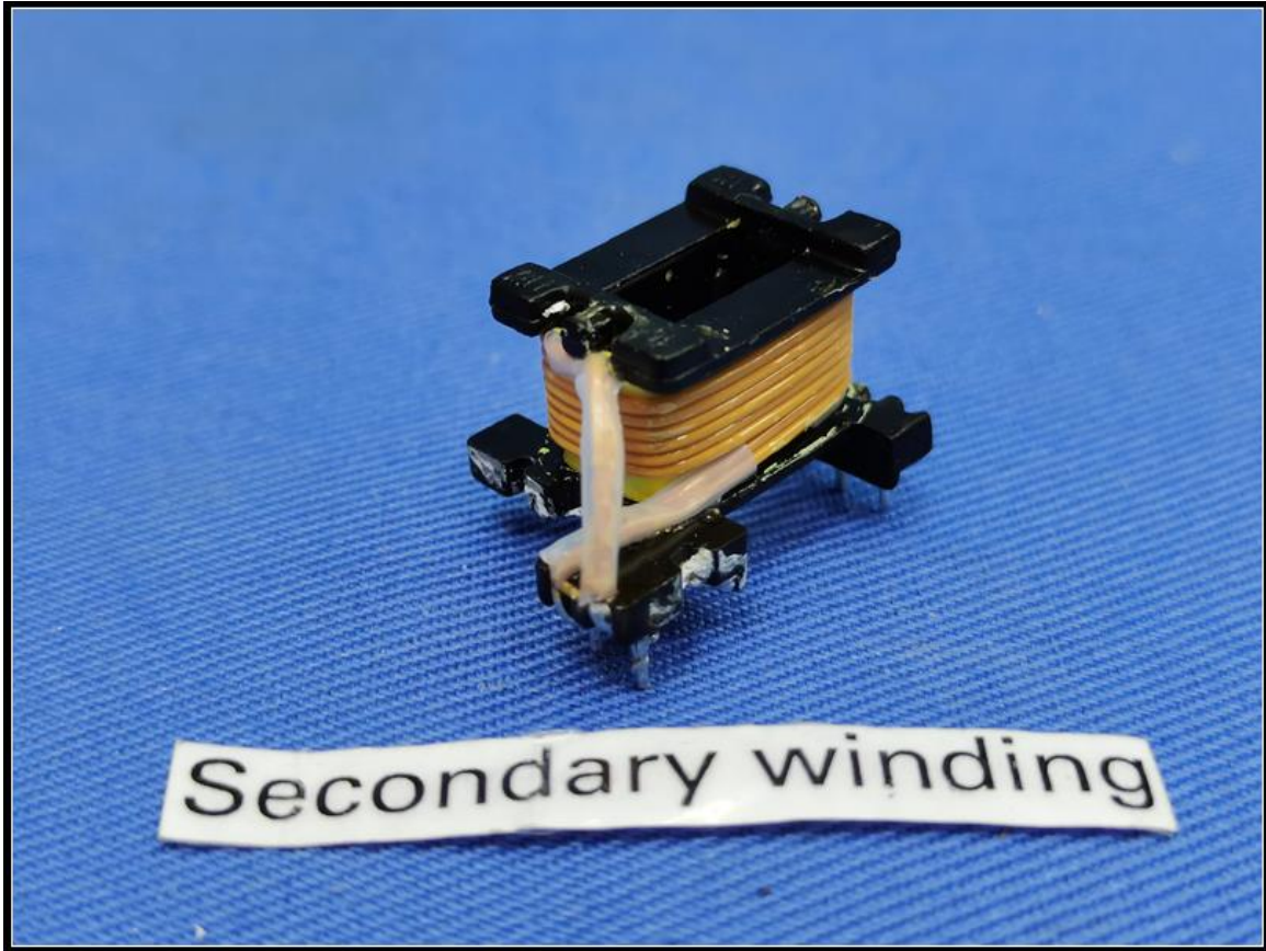
Insulation tube was used to separate primary winding and secondary winding
