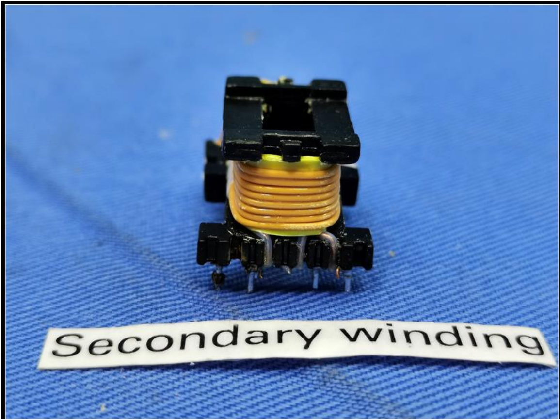
Insulation tube was used to separate primary winding and secondary winding
