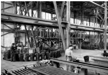
Carousel carrying upright sand moulds of about 1900
