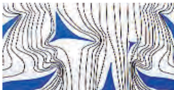
Path followed by the stress lines in cast iron with lamellar graphite (on the left) and with spheroidal graphite (on the right)
