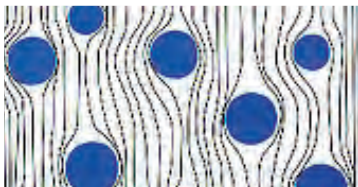
Path followed by the stress lines in cast iron with lamellar graphite (on the left) and with spheroidal graphite (on the right)
