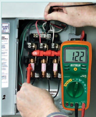
Accurate True RMS Voltage measurements on distorted waveforms
