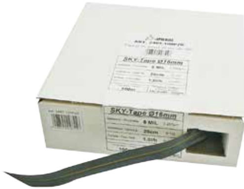
Tape Ø 16 mm 100 m pack, pitch 20 cm Rated flow-rate of each dripper 1.5 L/h Operating pressure between 0.4 and 1,2 bar
