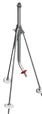
Galvanised iron tripod thread. 1" M and thread.adaptor 3/4" M Inlet with Ø 25 mm barbed connector Height-adjustable from 60 to 80 cm
