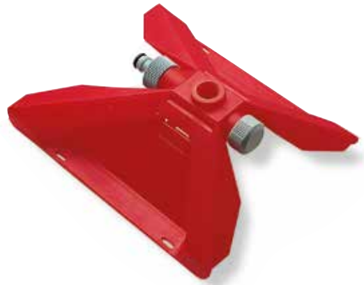
Sled for sprinklers, inlet with M coupling or thread. 3/4" M Thread. outlet F 1/2" Allows in-series connection
