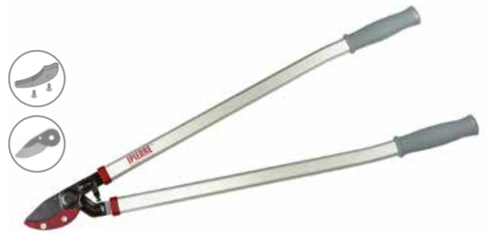
Ratchet anvil lopping shears, 80 cm, with Teflon-coated curved blade Anodised aluminium handles, blade in hardened carbon steel HRC 54:56
