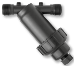
1" M - 1" M filter Filtering cartridge in 155 stainless steel Mesh (100 Micron) Maximum flow rate 80 l/min Maximum operating pressure 10 bar Body and plug in Nylon Drainage plug Ø 1/2" F for quick cleaning
